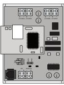
Repeater (optional) Supplied w/24 VAC transformer inside NEMA 1 enclosure (P/N 10080445)
